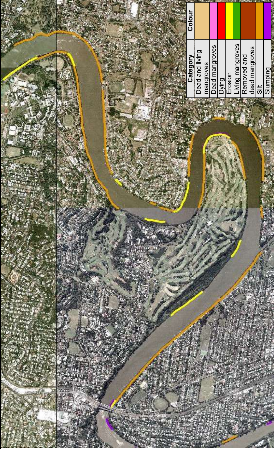
Aerial photograph 9 St Lucia to Walter Taylor Bridge, Indooroopilly showing silting, erosion and slumping February 2011.
