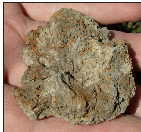
Figure 2. Ferruginous root channel linings provide reliable evidence of plant growth in a saturated environment, where the root has pushed oxygen into the saturated soil forming a coating of ferric iron around the root channel
