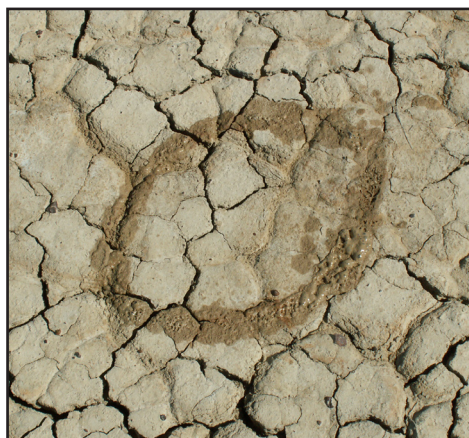
Figure 1. A strong reaction from a hydrogen peroxide field test for sulfidic materials
