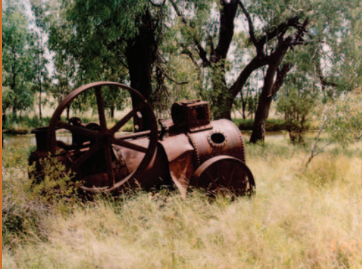
Steam traction engine used to power a portable sawmill (using coolabah trees). Photo: David Cameron
